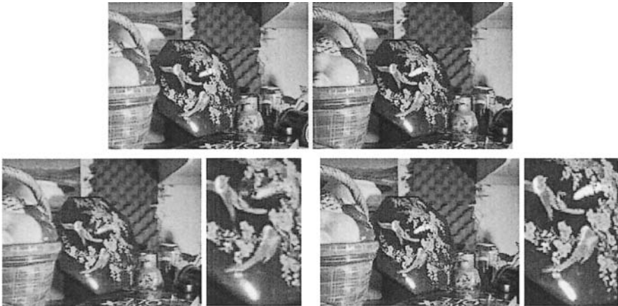
Fig. 2.24. Importance of view-dependent texture and geometry. Depth maps were extracted with the source images as reference views using the multi-view stereo technique described in [140]. Top: Source images. Notice the significant changes in the highlights. Bottom: Interpolated (left) vs. actual (right) views, with close-ups of the highlights. The highlights are a little blurred in the virtual view but resemble the actual version.
