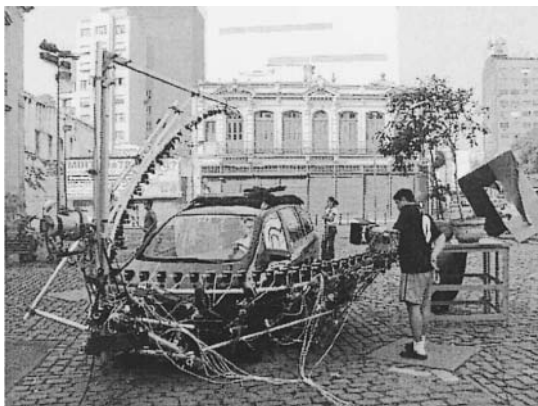
Fig. 3.2. Movia digital camera system (photo taken in April 2003). The 36 cameras are synchronized and saved uncompressed directly to digital disk recorders. The frame resolution is 1024 \times 768 and the capture rate is 15 fps. Photo courtesy of Digital Air.
