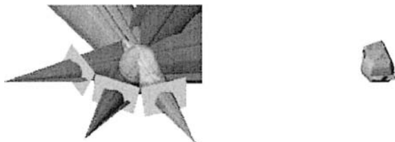
Fig. 3.9. Three extruded silhouettes of a teapot (left), and the resulting visual hull (right). (Figure courtesy of Wojciech Matusik.)
