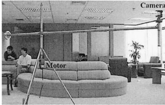
Fig. 2.7. Camera setup for acquiring Concentric Mosaics (CMs). The camera is counterbalanced by a weight; during image acquisition, it is rotated by a motor at a constant rotational speed.
