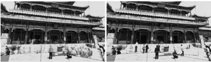
Fig. 2.14. Graph-based deghosting [303]. Left: Without deghosting. Right: With deghosting. Images (courtesy of Matthew Uyttendaele) are from “Eliminating ghosting and exposure artifacts in image mosaics,” by M. Uyttendaele, A. Eden, and R. Szeliski, IEEE Conference on Computer Vision and Pattern Recognition , Dec. 2001, vol. 1, pp. 2-9. ©2001 IEEE.
