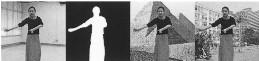
Fig. 12.20. (a) Input image (left). (b) alpha map. (c)-(d) New images of compositing extracted foreground over other background scenes.
