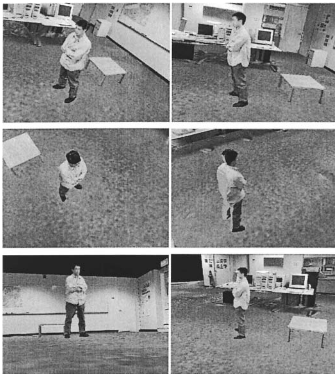
Fig. 3.11. Rendered IBVH at different views. The back of the person was unseen by any camera, which accounts for the missing texture (right image in middle row). Used with permission (courtesy of Wojciech Matusik).
